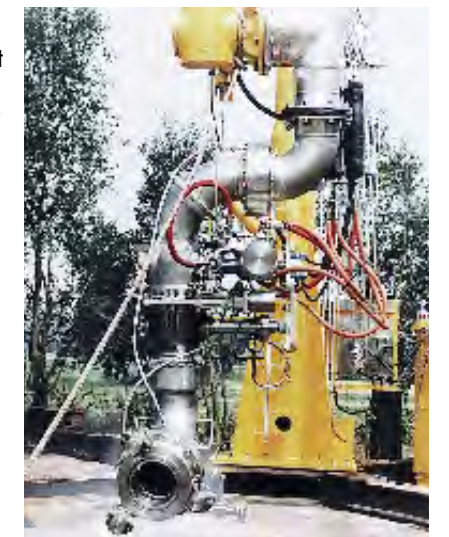
An industrial installation is shown above. RITE CAMLOCK COUPLINGS allow the user to rapidly disconnect the hose from the storage tank and connect it to another. Also the hose can be connected with a RITE CAMLOCK COUPLING to the pump as shown below.
